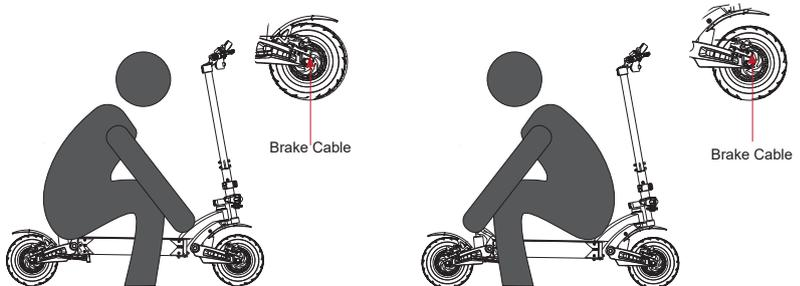
If the brake is too tight, pls use M5 hex wrench to loose the screw of the disc brake holder by anticlockwise direction, and short the brake cable, then fix the screw tightly; if the brake is too loose, just loose the screw and make the brake cable to be longer and then fix the screw tightly.
