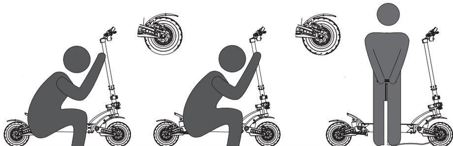
If the main rod shakes during the running, please tighten the nuts for clamp and secure it.
