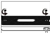
1. Unscrew the pedal cover screw counterclockwise.
