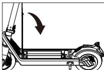
3. Cover the pedal and fasten the silicone edge of the pedal.
