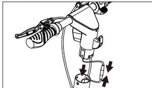
2. Align the communication line terminals of the instrument and the controller with the notch connection.
