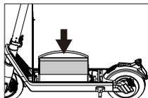
1. Put the battery vertically into the scooter.
