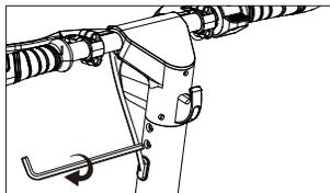
3. Align the T-bar of the scooter then insert it into the pole, use the screw provided with the scooter to install and fix it.
