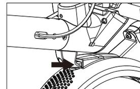
4. Gently press down the hook to the rear baffle.
