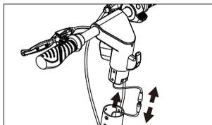
2. Pull out the head of the scooter, unplug the communication line between the display and the controller, the dismantling part of the head of the scooter is complete.
