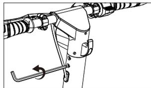
1. Loosen the screws that secure the T-bar of the scooter.
