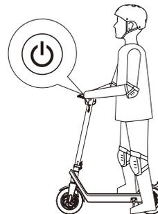
2. Long-Press the power button to turn on scooter, stand on the pedal with one foot, press the accelerator, and push the other foot back on the ground.
