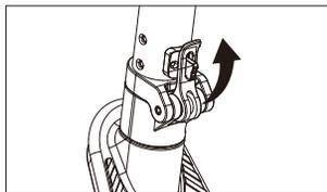
1. Unfold the pole and fasten the folding lock.
