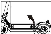
2. Lift the pedal cover from the quick-release screw on the rear wheel side.
