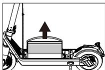
4. Lift the battery strap and take out the battery.
