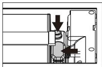
2. Connect the charging plug and the power plug of the controller to the battery.
