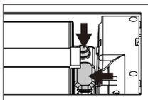
3. Unplug the charging plug and the power plug of the controller.
